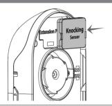
Install Knocking Sensor(KNS100) into extension port on PeepHole Viewer (PHV1330).
