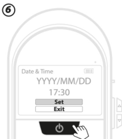
7. Press the **UP** and **DOWN** **BUTTON** to select the date and time. Then, press the **POWER BUTTON** to confirm.
