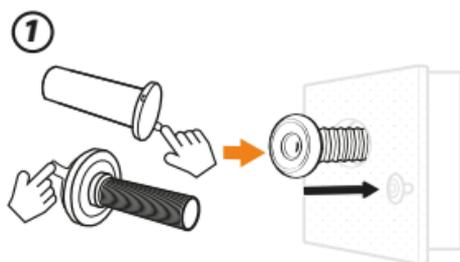
2. **For the 12mm Peephole** (For most North American users.) Position the Peephole barrel through the washer into the base flange from inside of the door. Tighten it.
